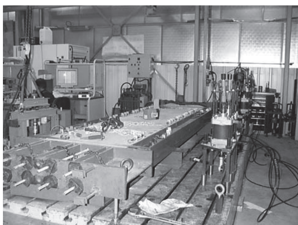
Equipment for testing in cracked concrete
